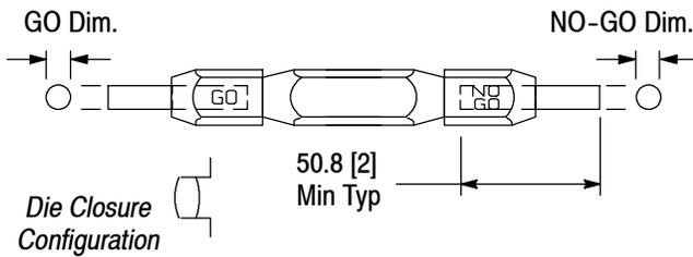
**Suggested Plug Gage Design for Insulation Barrel Section of Crimping Chamber**
