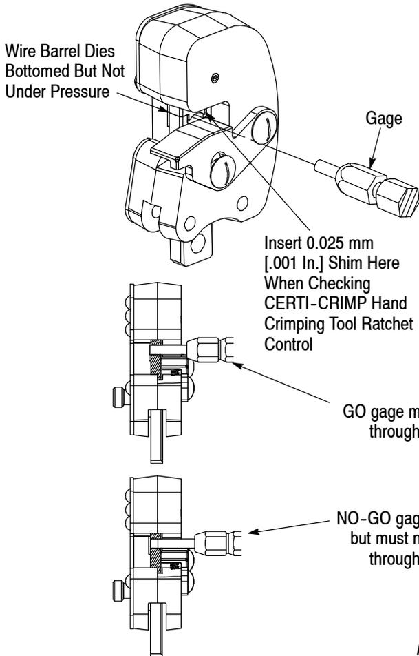
**(Detail B) Inspection of Insulation Crimping Dies**
