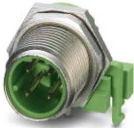
Bus system flush-type connector, ETHERNET, 4-pos., M12, shielded, D-coded, rear/screw mounting, with angled solder connection
