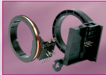
Orthocyclic wound coil with Multispring-Pressfit PCB-connection technology and R-welded wire-connection technology
