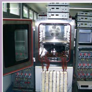
Test setup for fuse and relay box, combined static and electric load testing
