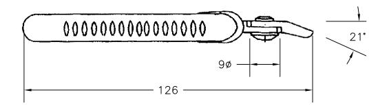
Notes: Cutting Capacity 2mm (12AWG) Soft Wire
