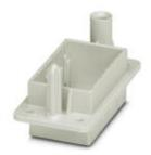
Docking frame for four module slots, fixed assembly, plastic without PE, rack compensation of +/-2.0 mm in the x/ y-axis, for M4 cylinder head screws
