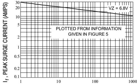
Fig. 6-PEAK SURGE CURRENT VERSUS PULSE WIDTH(SEE NOTE 3)
