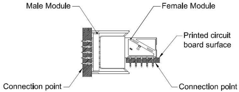
**Figure 3: Points of connection for contact resistance measurement.**
