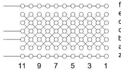
**Figure 4: Wiring arrangement for voltage proof.**
