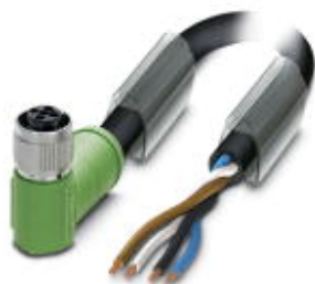
Power cable, 4-position, PUR halogen-free, black-gray RAL 7021, free cable end, on Socket angled M12 SPEEDCON, T-coded, Cable length: 2 m, for direct current up to 12 A/60 V
