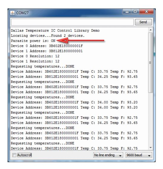
You'll also see the device addresses, these are the unique 64-bit addresses for each sensor. You have a promise from Maxim that they will never recycle these numbers! All **MAX31850** sensors start with **3B** which is the family address. You can see the temperature printed out afterwards
