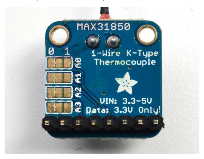
. You can solder the jumpers on the back but we'll be showing wiring with colored wires. In this case, we connect A2 to 3V and the rest to ground, That will make a binary address of 0100 = 0x4
