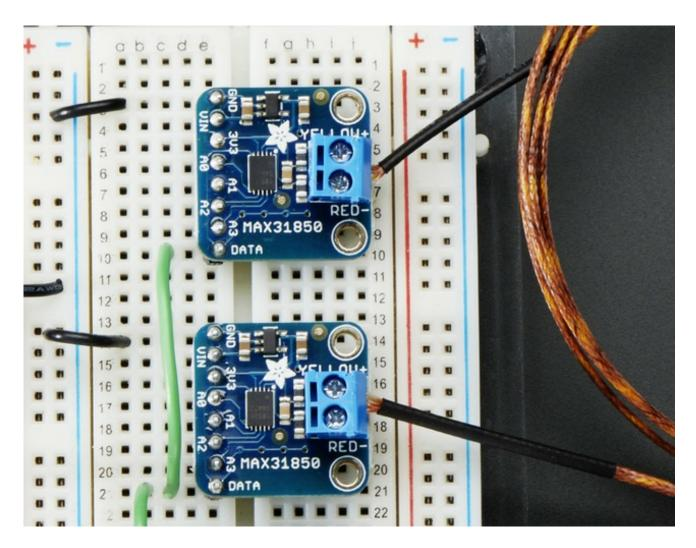
The MAX31850K data format is very similar to that of the well known 1-Wire DS18B20 temp sensor but it is *not drop in compatible* without code changes to check for the new '1 Wire family' type. We have adapted the classic Arduino OneWire (http://adafru.it/dal) and DallasTemp (http://adafru.it/dam) libraries to be MAX31850 compatible, so please click on those links to grab our libraries.
