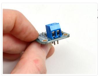
The terminal block goes on the top with the open ends pointing out
