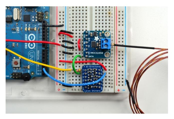
Now if you open up the serial console you should see the OneWire example code print out the data, address and temperature of the sensor. If you mess with the  $\mathbf{Ax}$  wires you'll see this address value change from 0x00 to 0x0F. This can be a good way to deal with 'hot-swapping' in sensors with unique ROM addresses
