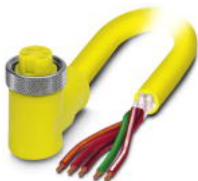
Sensor/Actuator cable, 5-position, PVC, Yellow RAL 1021, free cable end, on Socket angled 7/8"-16UNF, A-coded, Cable length: 2 m
