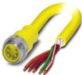
Sensor/Actuator cable, 5-position, PVC, Yellow RAL 1021, Plug straight 7/8"-16UNF, A-coded, on free cable end, Cable length: 4 m
