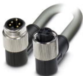
Power cable, 5-position, PUR, Gray RAL 7001, Plug angled 7/8"-16UNF, on Socket angled 7/8"-16UNF, Cable length: 1 m, 2.5 mm 2 conductor cross section, For power supply
