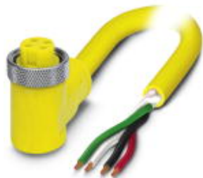
Sensor/Actuator cable, 4-position, PVC, Yellow RAL 1021, free cable end, on Socket angled 7/8"-16UNF, A-coded, Cable length: 2 m
