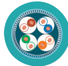
Cable cross section
