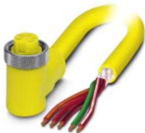
Sensor/Actuator cable, 5-position, PVC, Yellow RAL 1021, free cable end, on Socket angled 7/8"-16UNF, A-coded, Cable length: 6 m
