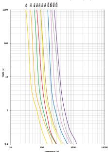
30 A - 150 A: FI = 1.25 (max. operating current:0.8 x  $I_{\rm rat}$  at 23°C) 200 A: FI = 2.00 (max.operating current: 0.5 x  $I_{\rm rat}$  at 23°C)
