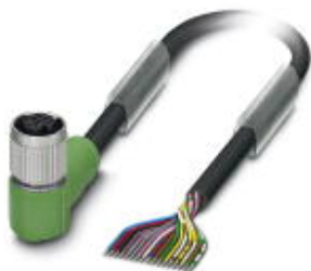
Sensor/Actuator cable, 17-position, PVC, Black RAL 9005, free cable end, on Socket angled M12 SPEEDCON, A-coded, Cable length: 3 m
