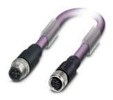
Bus system cable, PROFIBUS, 2-position, PUR halogen-free, violet RAL 4001, shielded, Plug straight M12, B-coded, on Socket straight M12, B-coded, Cable length: 14 m
