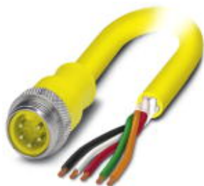
Sensor/Actuator cable, 5-position, PVC, Yellow RAL 1021, Plug straight 7/8"-16UNF, A-coded, on free cable end, Cable length: 6 m
