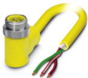
Sensor/Actuator cable, 3-position, PVC, Yellow RAL 1021, Plug angled 7/8"-16UNF, A-coded, on free cable end, Cable length: 6 m
