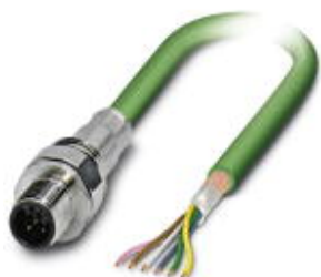
Bus system flush-type plug, INTERBUS, 5-pos., M12, shielded, B-coded, front/screw mounting with M16 thread, can be positioned, with 1 m bus cable, 3 x 2 x 0.25 mm 2
