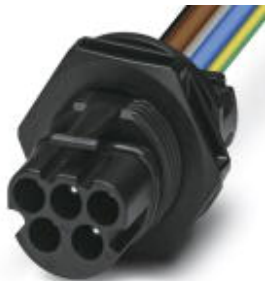
PRC device connector, black, 5-pos., 6 mm 2 /630 V/30 A, crimp connection, with 150 mm cable length, cut flat at the end
