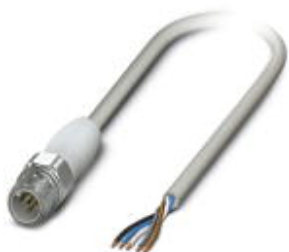
Sensor/Actuator cable, 5-position, PP-EPDM halogen-free, Gray RAL 7035, Plug straight M12, A-coded, on free cable end, Cable length: 1.5 m, Hygienic design, With high-grade steel knurl
