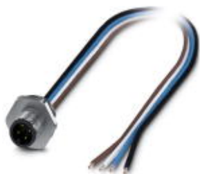
Bus system flat-type plug, PROFINET, 4-position, PlugLink:M12, D-coded, Front mounting, M16 x 1.5, Individual wires, Cable length: 0.5 m
