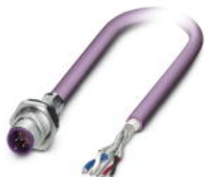
Bus system flush-type plug, DeviceNet/CANopen, 5-pos., M12, shielded, A-coded, SPEEDCON, rear/screw mounting with Pg9 thread, with 0.5 m bus cable, 2 x 0.2 mm 2 , 2 x 0.32 mm 2
