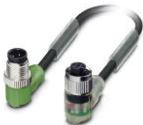
Sensor/Actuator cable, 4-position, PUR halogen-free, black-gray RAL 7021, Plug angled M12, A-coded, on Socket angled M12, A-coded, with 3 LEDs, Cable length: 3 m
