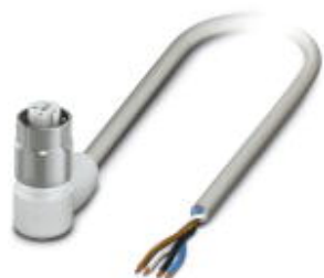
Sensor/Actuator cable, 4-position, PP-EPDM halogen-free, Gray RAL 7035, free cable end, on Socket angled M12, A-coded, with 3 LEDs, Cable length: 3 m, Hygienic design, With high-grade steel knurl
