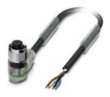
Sensor/Actuator cable, 4-position, PUR halogen-free, black-gray RAL 7021, free cable end, on Socket angled M12, A-coded, with 3 LEDs, Cable length: 1.5 m
