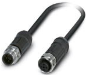
Sensor/Actuator cable, 4-position, PE-X halogen-free, black-gray RAL 7021, Plug straight M12, A-coded, on Socket straight M12, A-coded, Cable length: 2 m, for outdoor applications, With high-grade steel knurl
