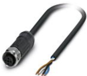
Sensor/Actuator cable, 4-position, PE-X halogen-free, black-gray RAL 7021, free cable end, on Socket straight M12, A-coded, Cable length: 5 m, for outdoor applications, With high-grade steel knurl
