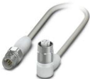
Sensor/Actuator cable, 5-position, PP-EPDM halogen-free, Gray RAL 7035, Plug straight M12, A-coded, on Socket angled M12, A-coded, with 3 LEDs, Cable length: 0.3 m, Hygienic design, With high-grade steel knurl
