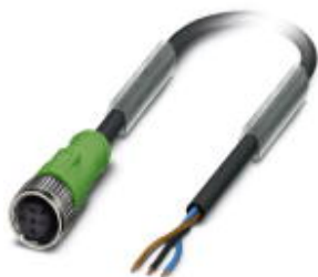
Sensor/Actuator cable, 3-position, PUR halogen-free, black-gray RAL 7021, free cable end, on Socket straight M12, A-coded, PIN 2+4 bridged, Cable length: 3 m
