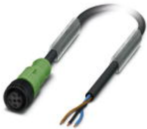
Sensor/Actuator cable, 3-position, PUR halogen-free, black-gray RAL 7021, free cable end, on Socket straight M12, A-coded, Cable length: 1.5 m, with plastic knurl
