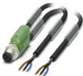
Sensor/Actuator cable, 3-position, PUR halogen-free, black-gray RAL 7021, Plug straight M12 SPEEDCON, A-coded, on free cable end and free cable end, Cable length: 1.5 m
