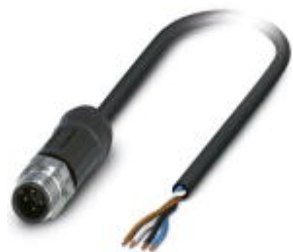
Sensor/Actuator cable, 4-position, PE-X halogen-free, black-gray RAL 7021, Plug straight M12, A-coded, on free cable end, Cable length: 2 m, for outdoor applications, With high-grade steel knurl
