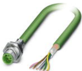
Bus system flush-type plug, INTERBUS, 5-pos., M12, shielded, B-coded, SPEEDCON, rear/screw mounting with Pg9 thread, with 0.5 m bus cable, 3 x 2 x 0.25 mm 2
