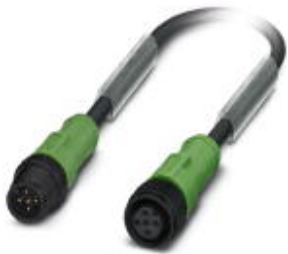
Sensor/Actuator cable, 5-position, PUR halogen-free, black-gray RAL 7021, Plug straight M12, A-coded, on Socket straight M12, A-coded, Cable length: 3 m, with plastic knurl
