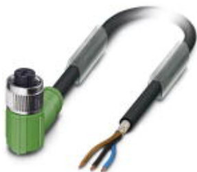
Sensor/Actuator cable, 3-position, PUR halogen-free, black-gray RAL 7021, shielded, free cable end, on Socket angled M12, A-coded, Cable length: 1.5 m
