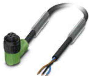
Sensor/Actuator cable, 3-position, PUR halogen-free, black-gray RAL 7021, free cable end, on Socket angled M12, A-coded, Cable length: 5 m, with plastic knurl
