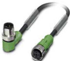
Sensor/Actuator cable, 3-position, PUR halogen-free, black-gray RAL 7021, Plug angled M12 SPEEDCON, A-coded, on Socket straight M12 SPEEDCON, A-coded, Cable length: 3 m
