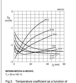
Fig.3 Temperature coefficient as a function o working current; typical values.
