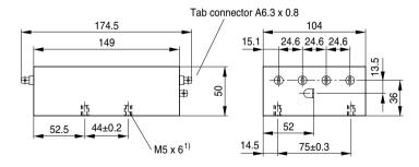
1) Also suitable for screws with 10-32 UNF thread
