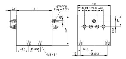
1) Also suitable for screws with 10-32 UNF thread
