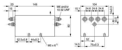
1) Also suitable for screws with 10-32 UNF thread
