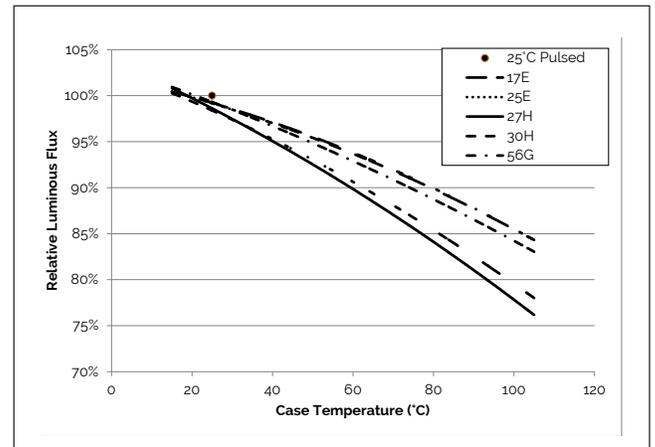
**Figure 9: Typical DC ccy Shift vs. Case Temperature**
