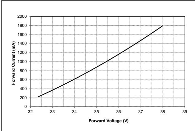
**Figure 2: Vero SE 18C Drive Current vs. Voltage**
