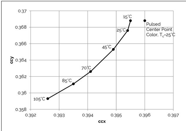
**Figure 18: 4000K Class A Color Shift vs. Case Temperature<sup>1</sup>**
