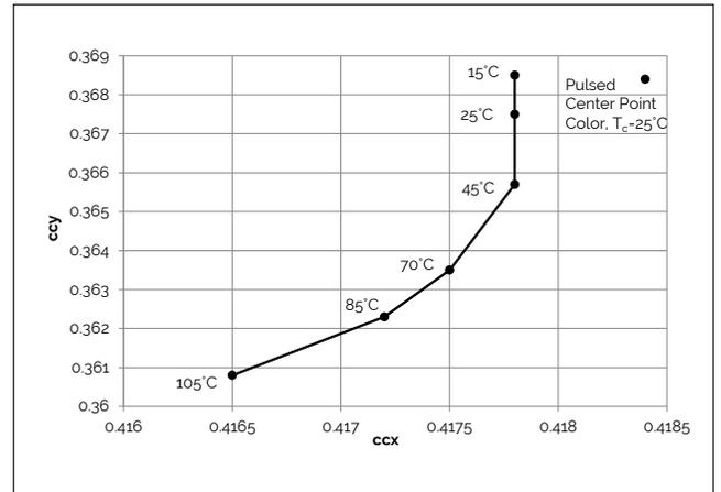
**Figure 17: 3500K Class A Color Shift vs. Case Temperature<sup>1</sup>**
