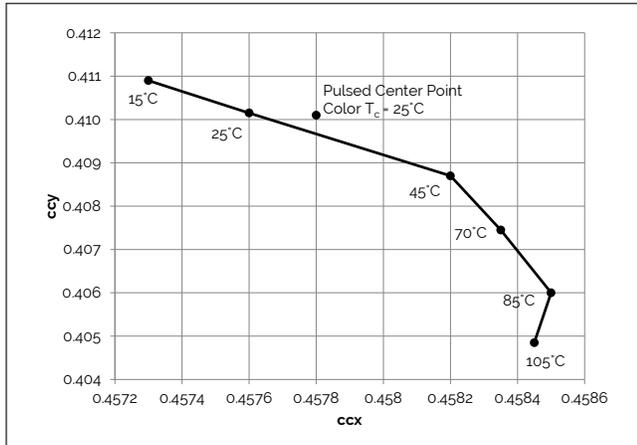
**Figure 14: 3000K, 97 CRI Color Shift vs. Case Temperature<sup>1</sup>**
