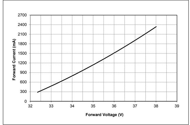
**Figure 3: Vero SE 18D Drive Current vs. Voltage**
