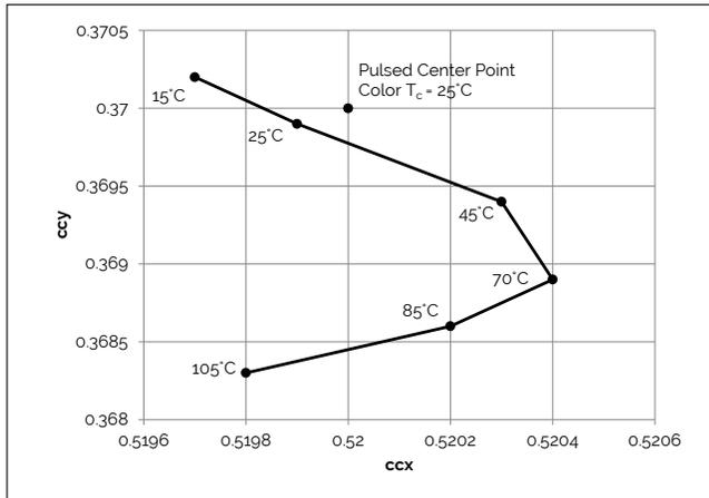
**Figure 12: 2500K Color Shift vs. Case Temperature<sup>1</sup>**
