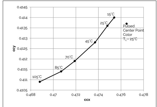
**Figure 13: 2700K, 97 CRI Color Shift vs. Case Temperature<sup>1</sup>**
