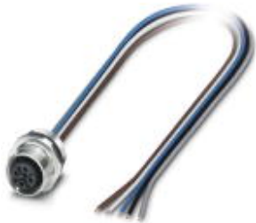
Sensor/actuator flush-type socket, 5-pos., M12, A-coded, front/screw mounting with Pg9 thread, with 0.5 m TPE litz wire, 5 x 0.34 mm 2 , stainless steel version
