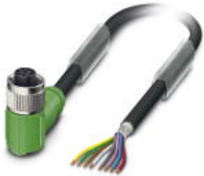
Sensor/Actuator cable, 8-position, PUR halogen-free, black-gray RAL 7021, shielded, free cable end, on Socket angled M12, A-coded, Cable length: 5 m
