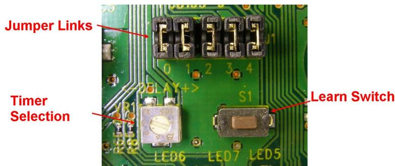
The jumper links configure the outputs to be Momentary, Latching or Timed. The jumper links are made / removed by a small link 'cap' placed over the pin header.
