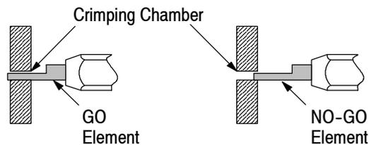
GO element must pass completely through the crimping chamber.
