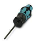
Torque screwdriver, with preset torque of 2.5 Nm and 4 mm hexagonal drive for the pressure nut of the connector hood
