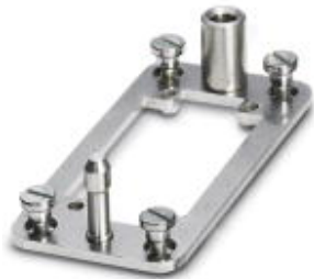
Docking frame for racks, for contact inserts of B10 type, with four M5 flat headed screws, rack balance x/y axis +/- 1.5 mm
